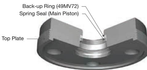
**Figure 30: Top Plate Image with Back-Up Ring**
